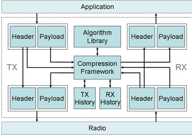
Fig. 3. Internal structure of the compression layer
