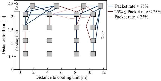
Fig. 1. Motes and communication links within a container with bananas (based on [10])
