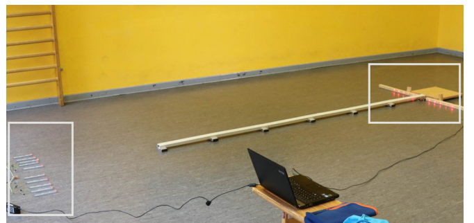
Fig. 8. Test setup with activated light barriers. Laser diodes are placed on the left; corresponding LDRs for detecting steps beside the beam located on the right. The notebook PC supplies power to the controller and laser diodes.
