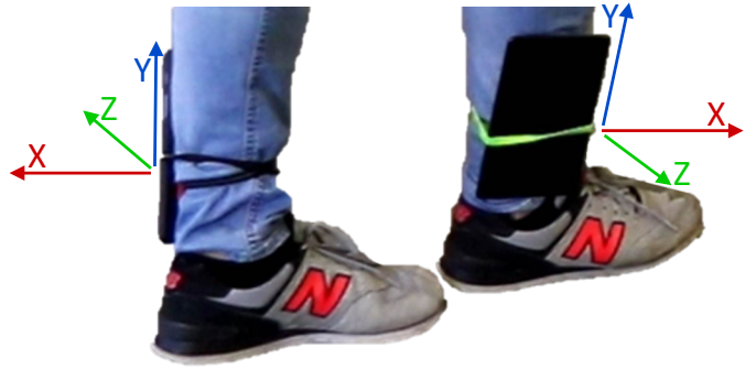
Fig. 4. Axis orientations of the gyroscope sensors mounted on a test subject’s lower legs. Note the inverted orientations of x-axis and z-axis between the devices due to their symmetric mounting.
