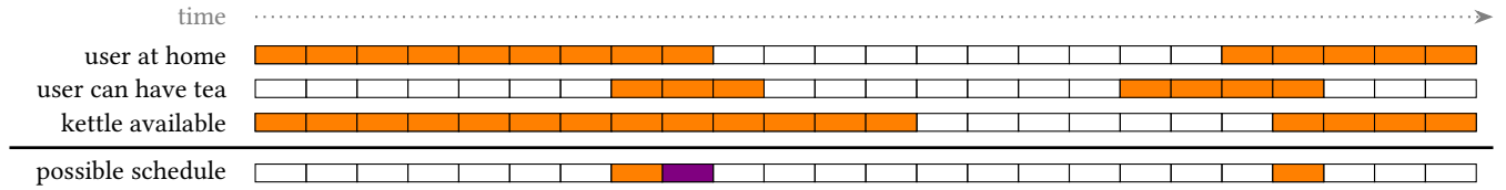
Figure 5: ANTgen internally relies on bitmaps to indicate user presence, activity times, and appliance usage. The logical conjunction of each bit is used to determine possible time slots at which an activity can take place.
