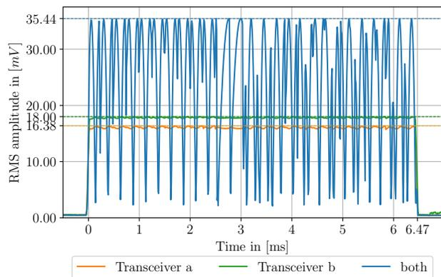
Figure 4. Analysis of the received RMS amplitudes for transceiver  $a$ ,  $b$  and the simultaneous transmission of both.
